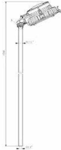
D — Lamp cap mounted in the angle of 25° fence type
